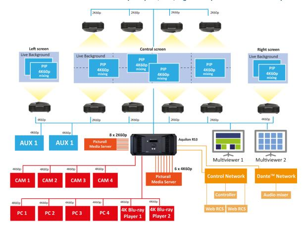
Aquilon RS3 can drive 2x 8K60p LED walls and 4x 4K60p AUX outputs
